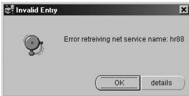
Figure 3-4. An Oracle Net Manager error message resulting from mapping more than one service name to a single connection descriptor
